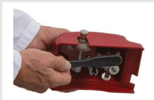
**6 Sharpening:** Press and hold the "A" button to bring the grinding stones in contact with the blade. Perform 20/30 blade rotations with the flywheel. Then release the "A" button and stop the rotation of the blade.
