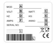
A =model of the machine B = Power supply C = power D = frequency E = Weight F = Amperes G = Year of manufacture / month of manufacture H = Serial number I = Manufacturer L = Barcode Fig. 1
