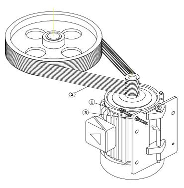
• Bowl drive belts may be adjusted by adjusting the screw nut No. 7 & 8.
