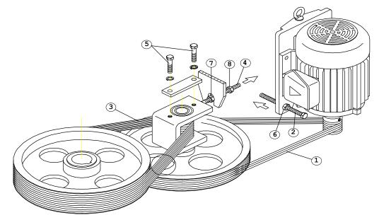
• Drive belts for the bowl drive motor may be adjusted by means of the screw No. 2 on lower motor support plate.
